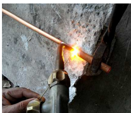
Figure 9. Brazing copper pipe.
