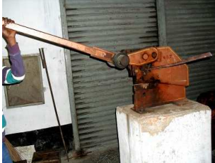
Figure 17. Processing steel plate in shear machine.
