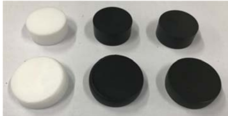
Figure 5. Before and after compression of test piece (from left to right are PTFE, 10C-PTFE, 20C-PTFE).
