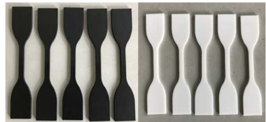
Figure 3. Tensile specimens.
