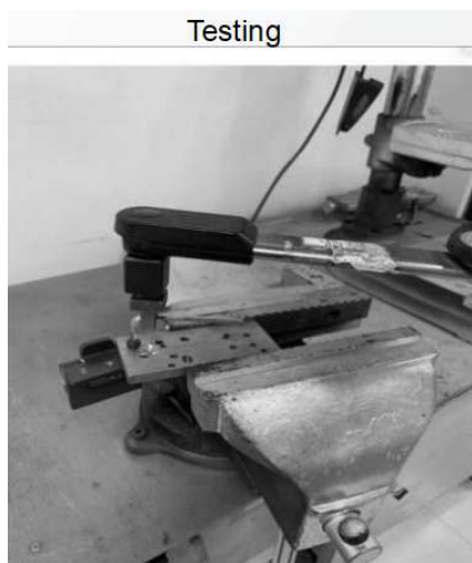
Figure 9. Torsion test of hinge.
