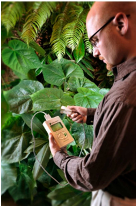
Figure 3. Steady state porometer measuring stomatal conductance.
