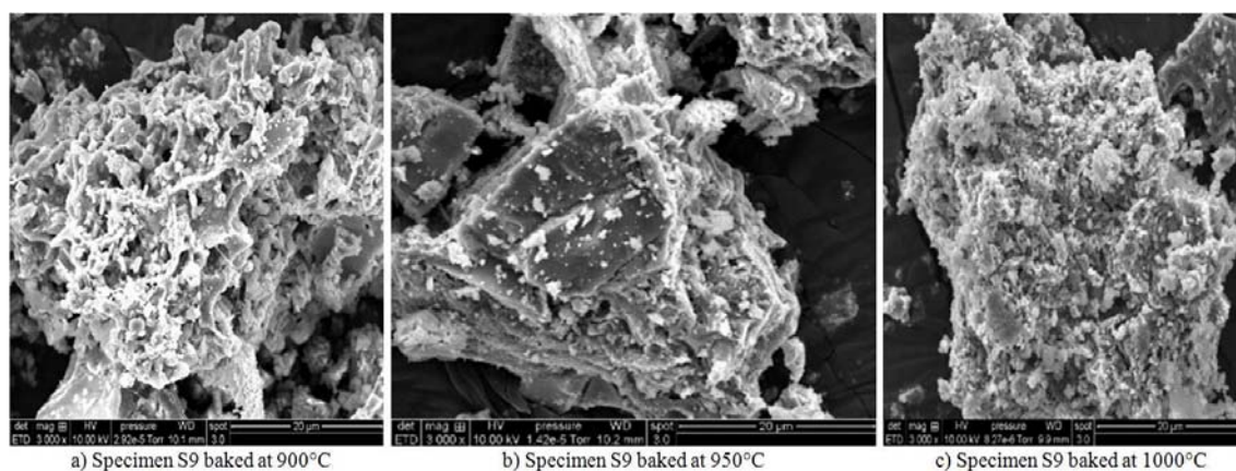
Figure 16. SEM images of S9 aggregates sintered at 900°C, 950°C and 1000°C for 30 min at 3000x magnification.
