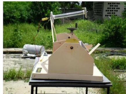
Figure 2. Solar Parabolic-Trough Collector (TE38).
