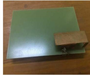
Figure 14. Experiments for PIFA Antenna.
