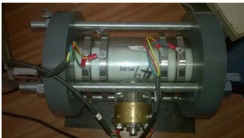
Figure 2. Plexiglass Pipe Test Tube with Ring Sensors and Probe Sensor.
