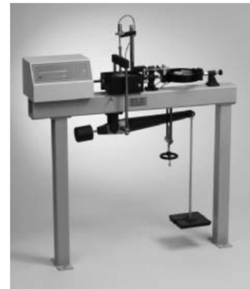
Figure 1. Figure shows a direct shear test equipment.
