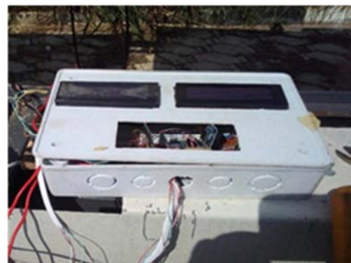
Figure 5. The final prototype of the proposed irradiance meter.
