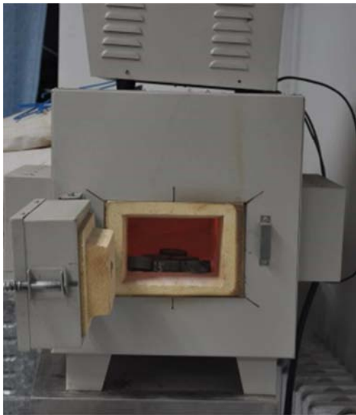
(a) Ceramic fiber resistance furnace
