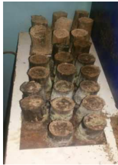
Figure 1. Briquettes (wet) immediately after extrusion from machine.
