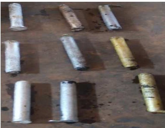
Figure 3. Quenched samples in water, palm oil, and engine oil.
