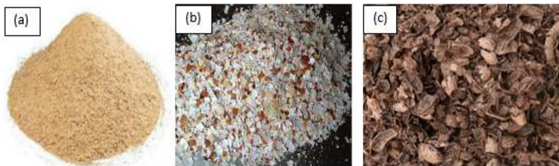
Figure 1. Sand mould additives: (a) sawdust (b) egg shell and (c) groundnut shell.
