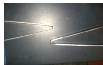
Figure 7. Test Specimens showing satisfactory weld properties.
