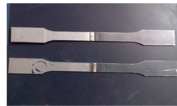
Figure 4. Tensile Test Specimens.
