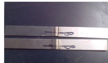
Figure 5. Test specimens for bend tests.
