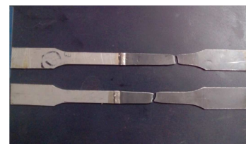
Figure 6. Test Specimens showing failure at CS side away from weld and HAZ.
