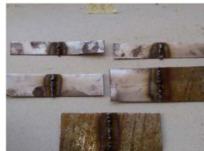
0.8 mm Welded Mild Steel Plate Specimen
