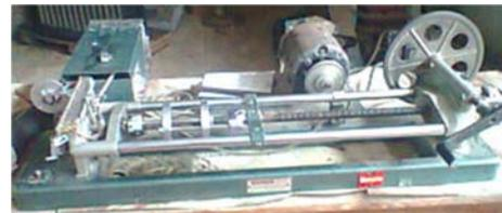
*Figure 2. Brinell Hardness Testing Machine.*
