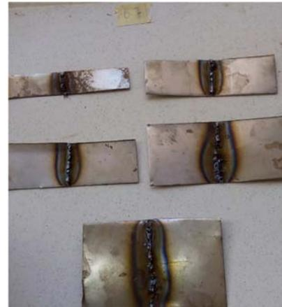
0.7 mm Welded Mild Steel Plate Specimen
