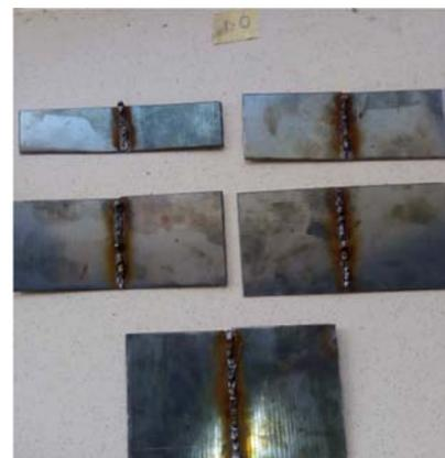
1.0 mm Welded Mild Steel Plate Specimen
