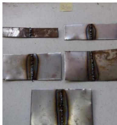
0.6 mm Welded Mild Steel Plate Specimen
