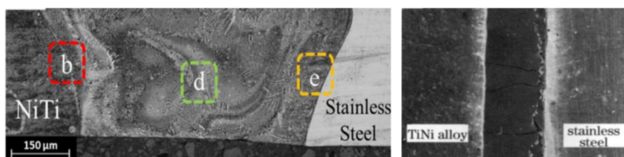
Figure 3. Microstructure of the weld zone when the laser is focused on the center line (left).
