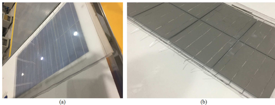
Figure 3. Optical images of solar panels encapsulated by PC (a) the front (b) back.
