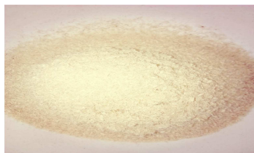
Figure 3. Sodium hydroxide modified Kenaf fiber.
