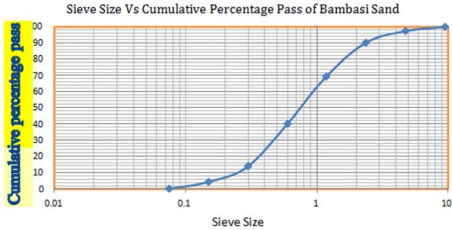
Figure 3. Grain Size Analysis Aggregate result of Bambasi sand.
