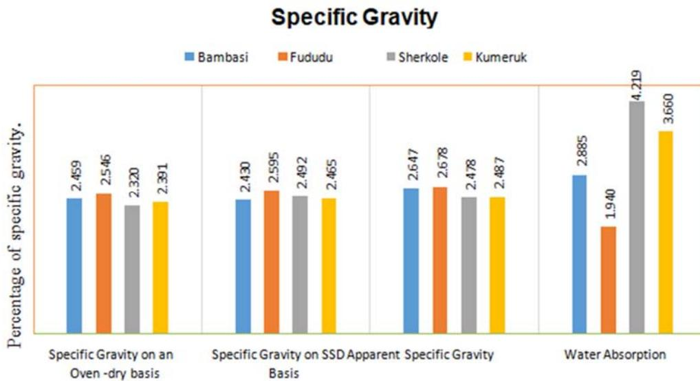
Figure 10. Specific Gravity and Water absorption of sands.
