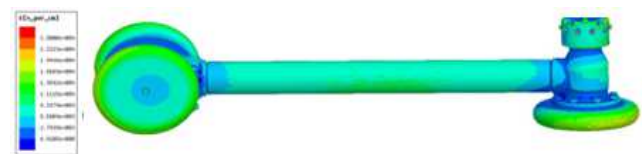
Figure 9. Insulator Top Flange Shielding (round current path arm of a center break disconnector with vertical contact system shielding, 420 kV application).
