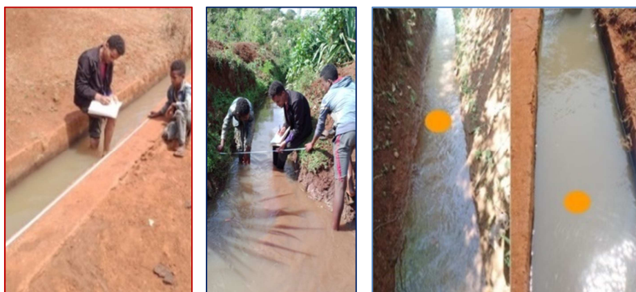
Figure 2. Discharge measurement by area-velocity method.
