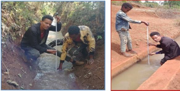
Figure 3. Water surface elevation measurement.
