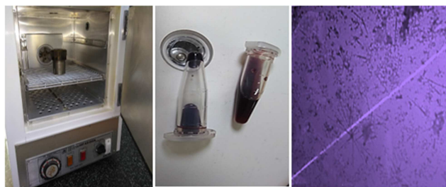
Figure 1. Photographic images of MOF synthesis (a)- Reactants put in hydrothermal bomb, (b)- 0.2 mg precipitate taken for centrifuge @8000 rpm. (c)- Ultra microscopic image of MOF".
