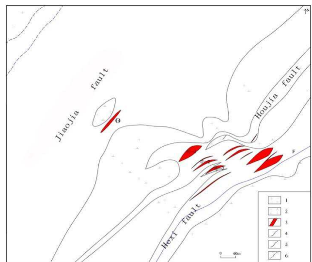
Figure 4. Map of underground vein distribution in Xincheng gold mining area.
