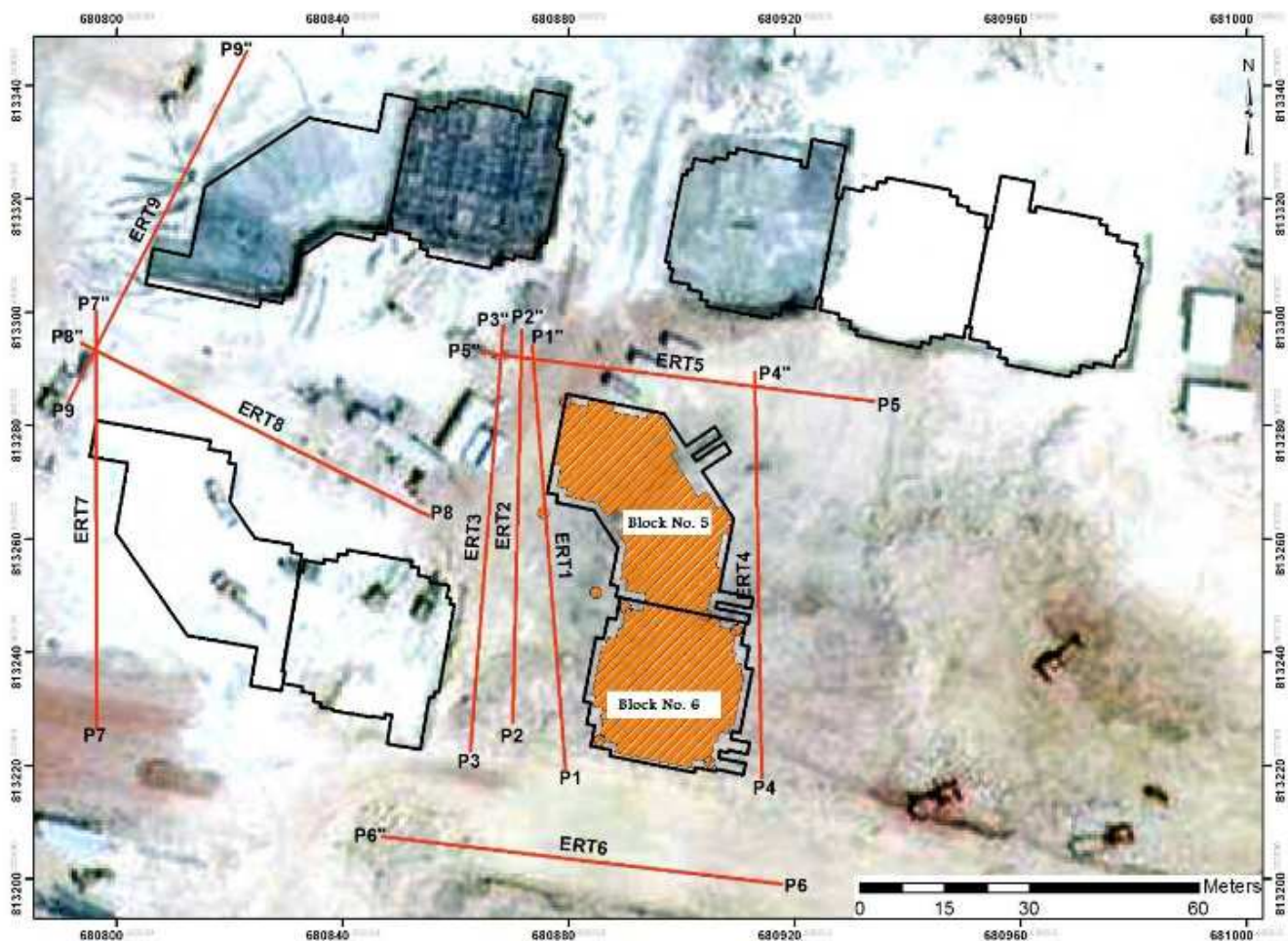
Figure 4. Spatial distribution of the measured ERT Profiles.
