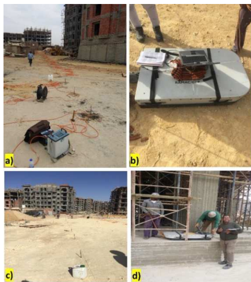
Figure 3. Documenting the field measurements and Devices a) [23] instrument and its accessories, b) [24] GPR and its accessories, c) the distribution of electrodes array in survey of ERT profile no. 7, d) survey of GPR profile 14.
