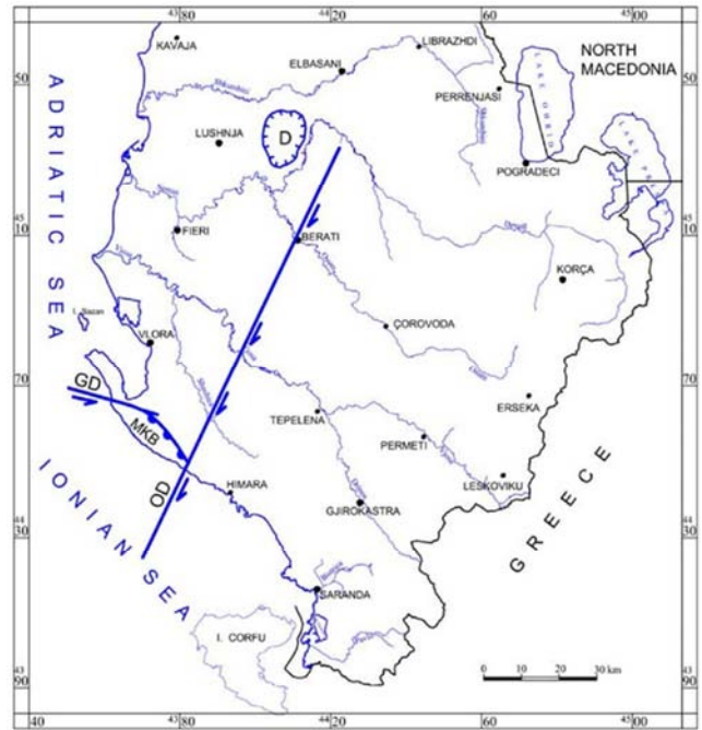
Figure 7. The offset of Devolli (to the east of Dumre diapir), Osumi (near to Berati town), and Vjosa (west of Shkoza village) river's valleys is due to the dextrally dragged Othoni Island-Dhermi strike-slip fault. D- Dumre diapir, OD-Othoni Island-Dhermi dextral strike-slip fault and GD-Gjiri i Ariut-Dukat i Ri sinistral strike-slip fault bound the MKB-Mali i Kanalit Block backthrusting the Çika anticlinal belt of Ionian Zone.
