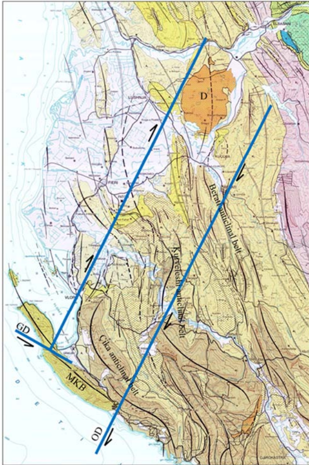
Figure 6. Tectonic Map of the Mali i Kanalit Block - Dumre diapir dextral strike-slip fault zone NNE trending in transpression that crosses the Albanides Ilision Zone in NE-SW compression. Map based on Tectonic Map of Albania in scale 1:200,000 [42]. The GD- Gjiri i Ariut - Dukat i Ri and OD - Othoni Island-Dhermi strike slip faults bound the Sazani Zone Mali i Kanalit Block (MKB) that backthrusts towards NNE the Çika anticlinal belt of Ionian Zone. D-Dumre diapir. The marked Çika, Kurveleshi and Berati anticlinal belts show their strong offset within the Mali i Kanalit Block-Dumre diapir strike-slip zone.
