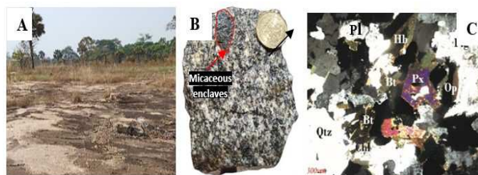
Figure 3. Macroscopic and microscopic aspects of granodiorite of Kakoubroukro (Kak01) Bt: biotite, Chl: chlorite, Px: pyroxene, Hb: green hornblende, Pl: plagioclase, Qtz: quartz.
