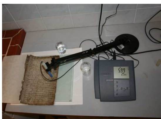
Figure 5. Measuring the pH value of the paper surface.
