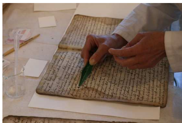
Figure 6. Identification of ink using indicators.
