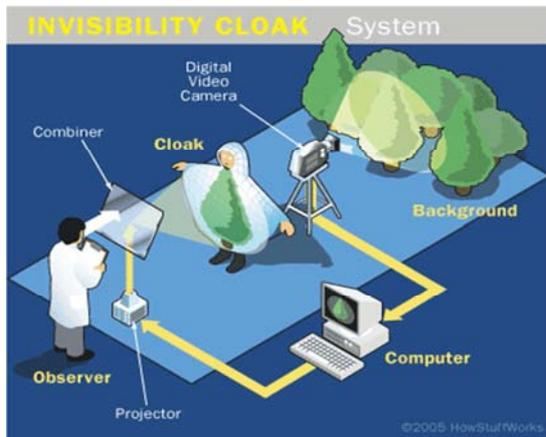
Figure 9. RPT System for active camouflage.
