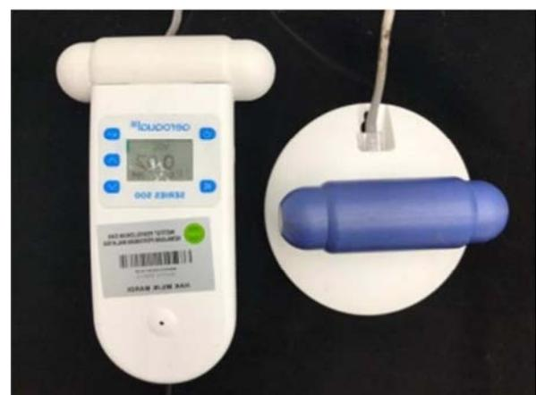
Figure 2. Gas detector (model Aeroqual S500).
