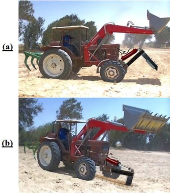
Figure 4. The horizontal penetrometer mounted on the tractor in field: a) penetrometer outside the soil and b) penetrometer inside the soil.
