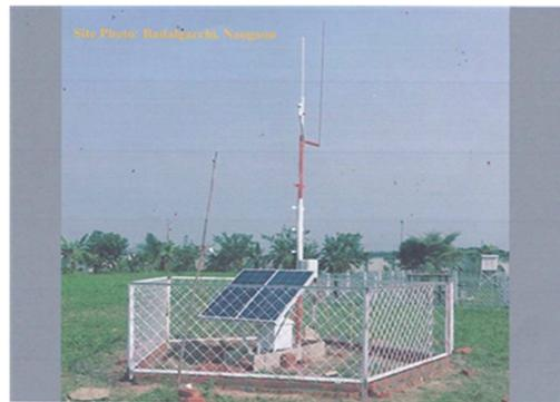
Figure 3. Installed Lightning detector in Bangladesh.
