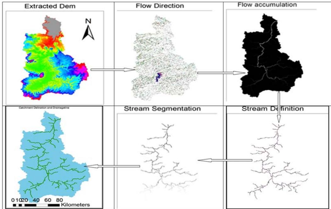
Figure 3. HEC-GeoHMS Terrain Processing of Dabus sub basin.
