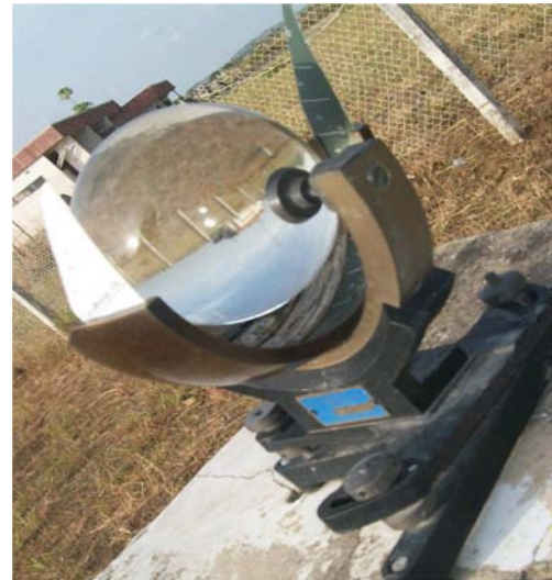
Figure 11. Sun-shine recorder instrument.
