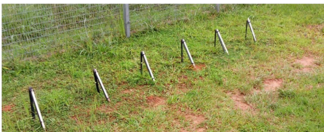
Figure 2. Soil thermometers at NIMET, Enugu.
