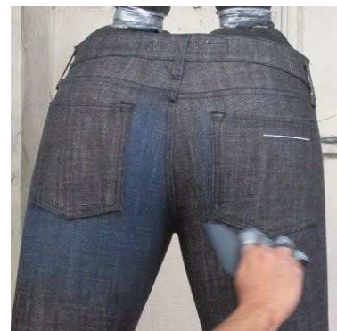
Figure 4. Hand sand on back part area of stretch denim.
