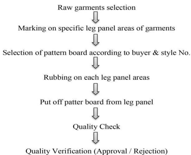
Figure 3. Operational flow chart of manual whiskering
