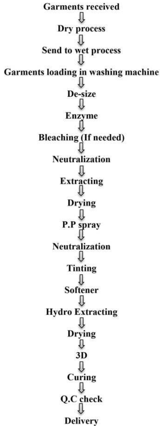
Figure 13. Operational flow chart of garments wet process.
