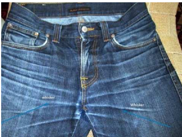
Figure 2. Sample manual whiskering
