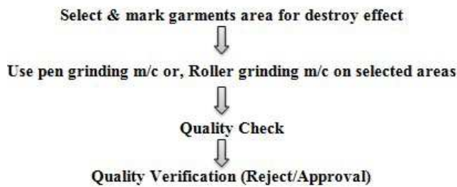
Figure 9. Operational flow chart of destroy effect.
