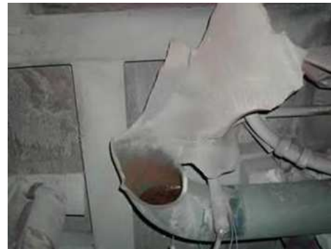
Figure 18. 2001 Hamaoka, Japan piping explosion due to water hammer (U.S. NRC)
