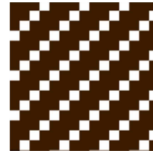
Figure 1. 3/1 twill fabric design RHT.
