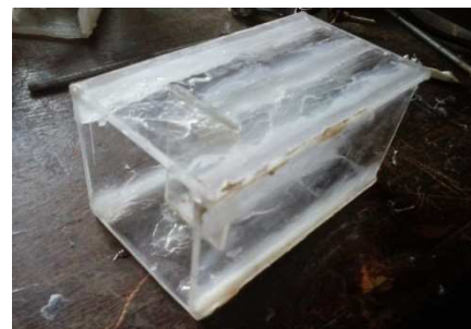
Figure 5. Case and inner separator having silicon seal applied to its corners and joints.
