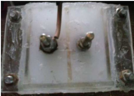
Figure 6. Top view of cell showing the electrodes cover and the applied silicon seal.
