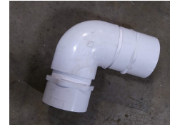
Figure 6. Male thread x female thread short radius elbow (MPTxFPT 1).
