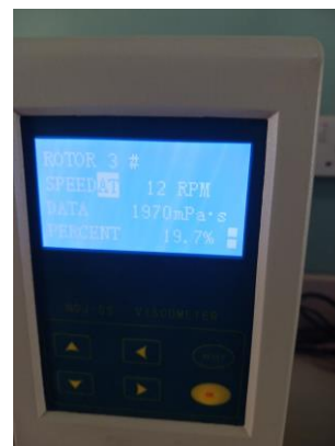
Figure 7. Shows a typical Viscometer reading at 12 RPM.
