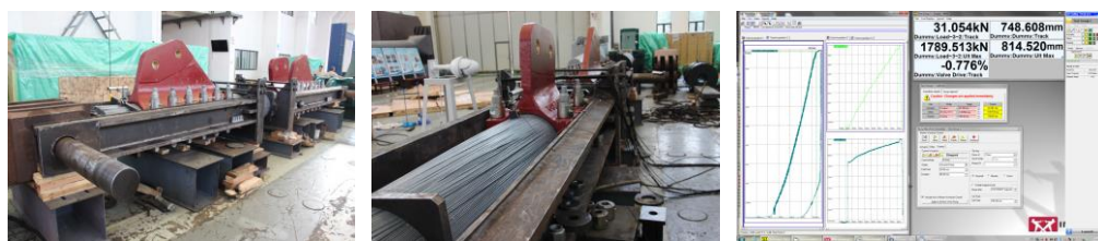
Figure 20. Anti-Slip Test Photo of Cable Clamp.
