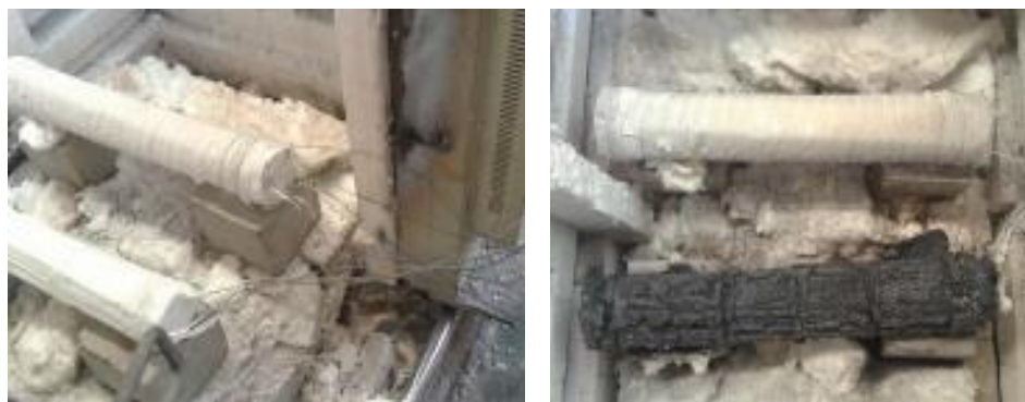
Figure 17. High-Temperature Testing of Thin-Film Fire-Resistant Coatings and New Ceramic Composite Insulation Wraps.
