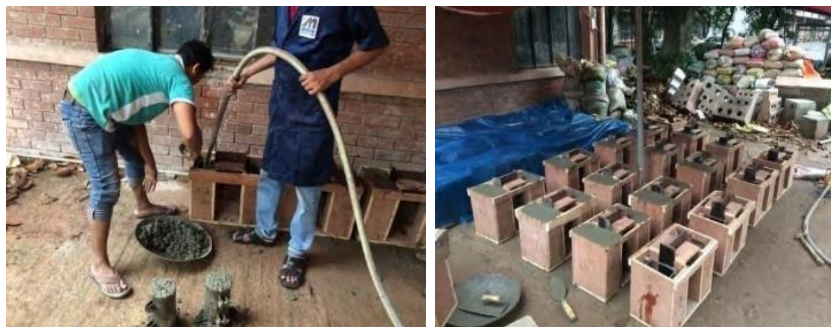
Figure 3. Push-out test specimen fabrication.
