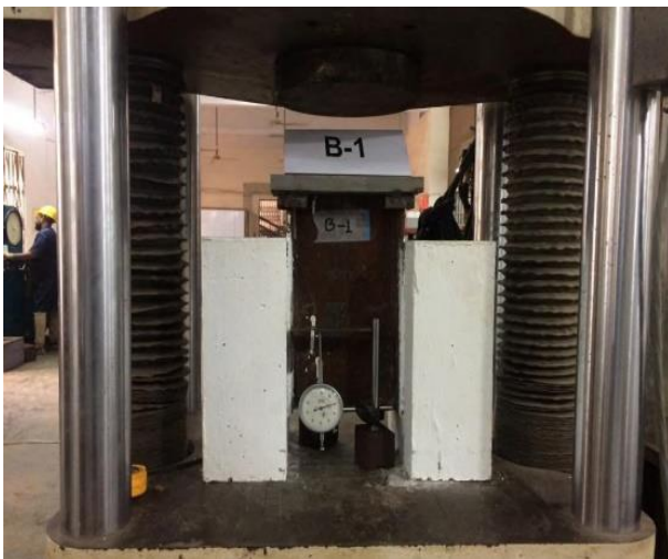
Figure 5. Typical Test Setup & Instrumentation.
