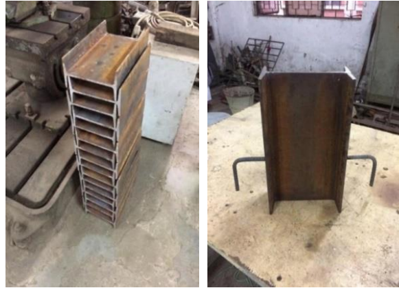
Figure 2. L-shape rebar connector attached to short steel beam.
