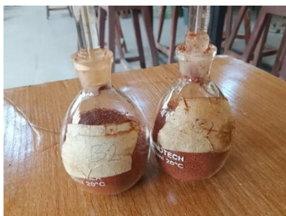
Figure 6. Sample in the Density Bottle (Pycnometer) with stopper.
