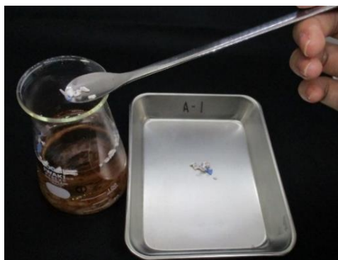
Step 5: Collecting light MPs
