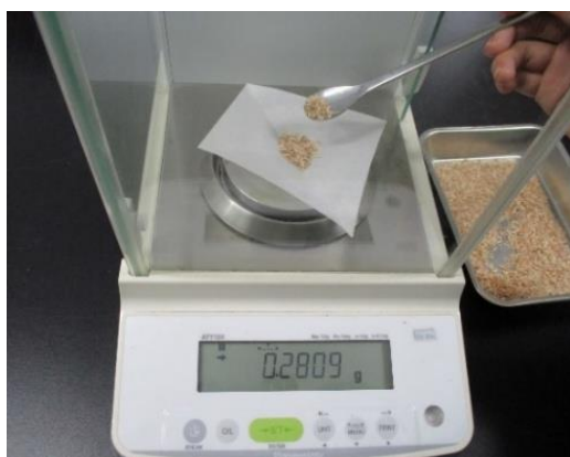
Step 1: Weighing samples
