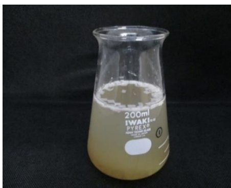
Step 8: Floating of heavy MPs
