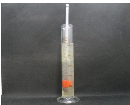
Step 12: Measuring SCC density
