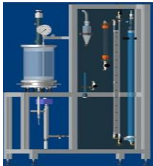
Figure 1. Batch Fluidized Bed Dryer.
