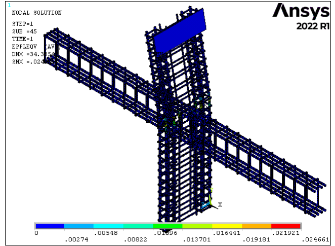
(b) 10 mm thick stiffener plate strengthened
