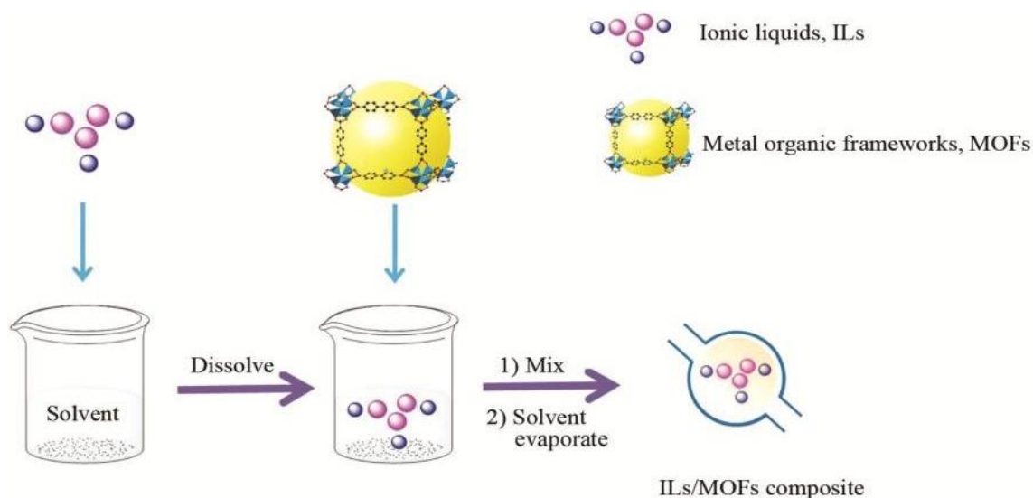
Figure 1. Wet impregnation technique schematic diagram for the impregnation of ILs into MOFs.
