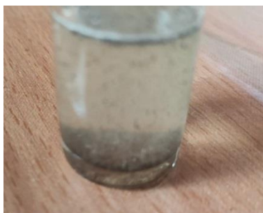
Figure 9. Formation of gas bubbles right from the start.
