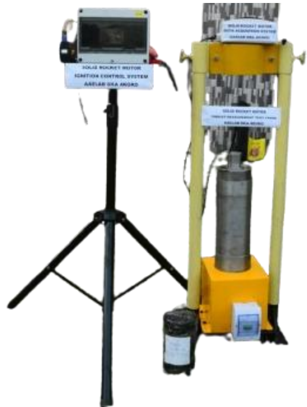
Figure 4. The Ignition system, the data acquisition system and the complete Test Stand.
