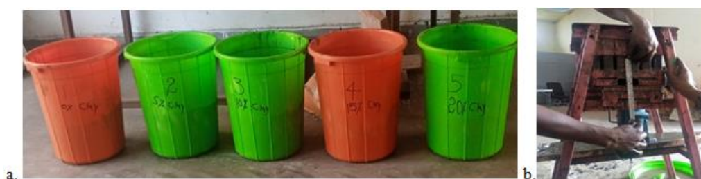
Figure 3. Treatment setup: factors of clay soil ratio (a) and factors of compression level (b).
