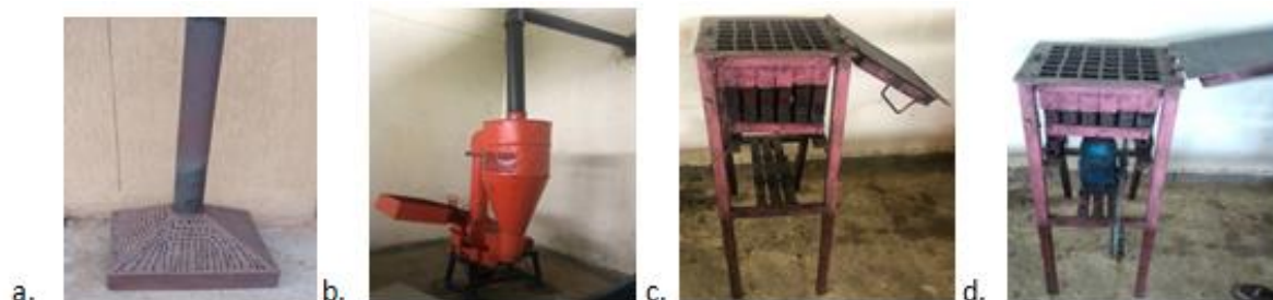
Figure 1. Components for Carbonized Rice Husk Briquetting Process, carbonizer (a), Hammer miller (b), mold maker (c), and mold maker with hydraulic jack (d).
