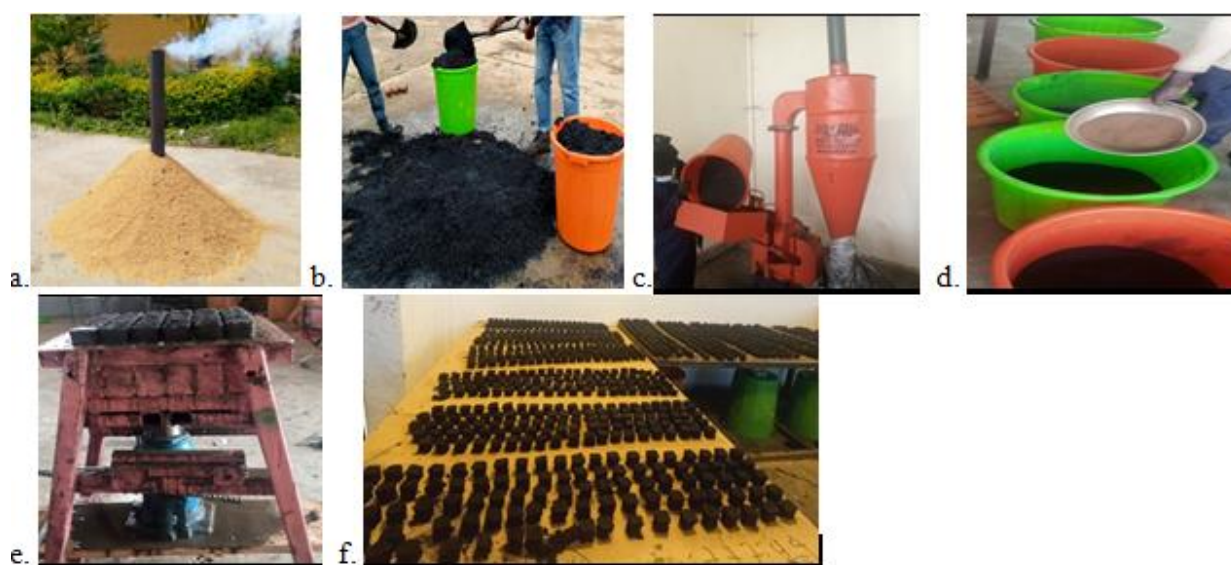
Figure 2. Process of carbonized Rice Husk Briquetting: Carbonizing of rice husk (a), cooling and storing of biochar (b), biochar grinding (c), mixing of biochar powder with clay and water (d), molding of the mix using mold maker and hydraulic jack (e) and biochar charcoal briquettes (f).
